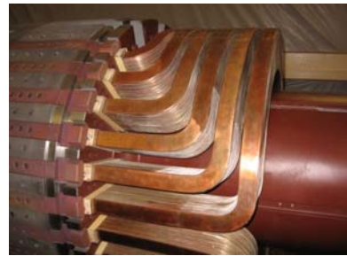
Rewound Coils Prior to Support Blocking Insulation
